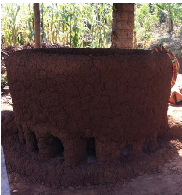
A Kiln for producing the Canarumwe stove
